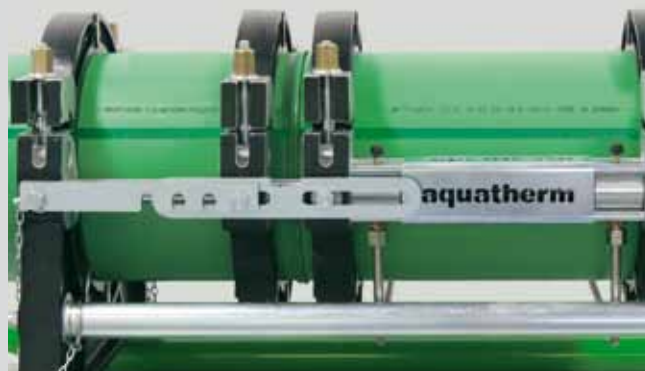
Join the pipes, cool down under pressure
